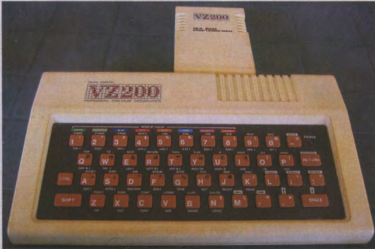
Above: The Dick Smith VZ200 sold over 25,000 inside two years, this one has the 16KB RAM expander (Image credit: I, John Dalton, CC-BY-SA 3.0)
