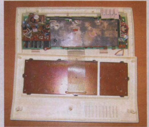
Above: The VZ200 was a very compact design, packed with chips and a Z80 CPU (Image credit: I, John Dalton, CC BY-SA 3.0).
