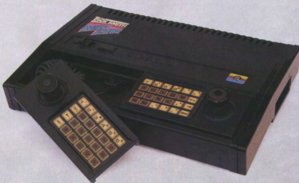
Above: The Dick Smith Wizzard combined 8-bit computer and games console (Image credit: Bilby, CC BY 3.0).
