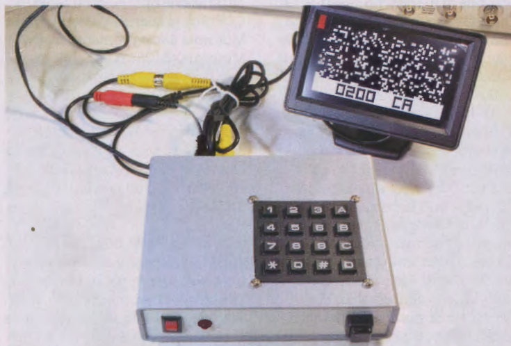
Above: I've designed a new 8-bit Arduino Nano-powered version of the DREAM 6800, here plugged into a 4.3-inch car LCD monitor (Image credit: Darren Yates).
